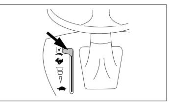
Figure 13. Combined Speed and Choke Control
